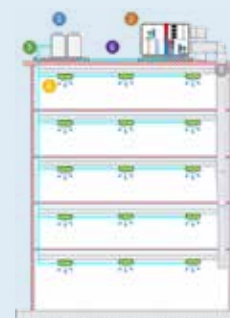
1 VRF 5 th Generation Heat Recovery Air Handling Unit 2 Air Handling Unit Fresh Air Ductwork 3 VRF Indoor Unit 4 VRF Indoor Unit Gas Piping 5 VRF - Air Handling Unit Gas Piping
