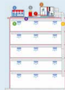
1 Chiller 2 5 th Generation Heat Recovery Air Handling Unit 3 Boiler 4 Air Handling Unit Fresh Air Ductwork 5 VAV 6 Chiller - Air Handling Unit Water Piping 7 Boiler - Air Handling Unit Water Piping
