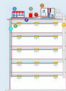
1 Chiller 2 5 th Generation Heat Recovery Air Handling Unit 3 Boiler 4 Air Handling Unit Fresh Air Ductwork 5 VAV 6 Chiller - Air Handling Unit Water Piping 7 Boiler - Air Handling Unit Water Piping 8 Chiller and Boiler - Air Handling Unit Water Piping
