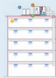
1 VRF 5 th Generation Heat Recovery Air Handling Unit 2 Air Handling Unit Fresh Air Ductwork 3 VRF Indoor Unit 4 VRF Indoor Unit Gas Piping
