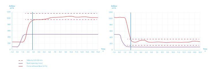
A sash sensor with a very quick reaction time ensures that the airflow is adjusted in less than one second (< 1 s) and the system is stabilised in less than three seconds (< 3 s). When the sash sensor has reached the desired level, the face velocity sensor takes over the control in order to maintain the velocity, taking also into account any blockage caused by people or equipment by the sash opening.
